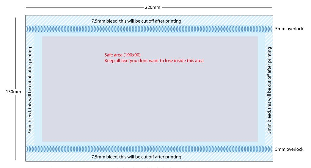
Please send files as JPEG or PDF 220x130mm, the bleed area is for the background only All text to fit within the 190x90 Safe area. allow 5mm top and bottom clearance for the overlocking.
